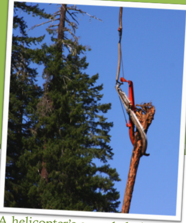
A helicopter's grapple holds a tree as it is lowered into position
