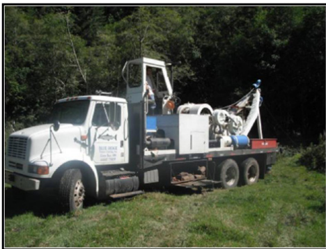
Truck-mounted cable yarder used to pull logs into place in Scholfeild Creek.
