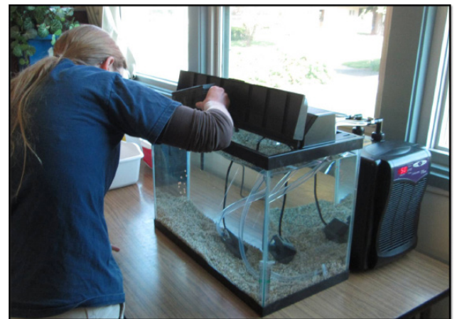
Amy Pinson-Dumm delivering eggs. To create a salmonid-egg-friendly environment, the water is circulated through the black chiller to the right of the fish tank.
